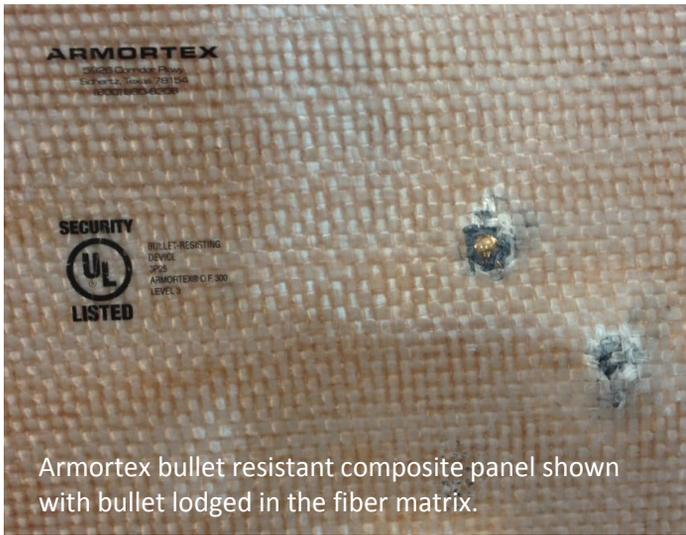
Armortex bullet resistant composite panel shown with bullet lodged in the fiber matrix.
